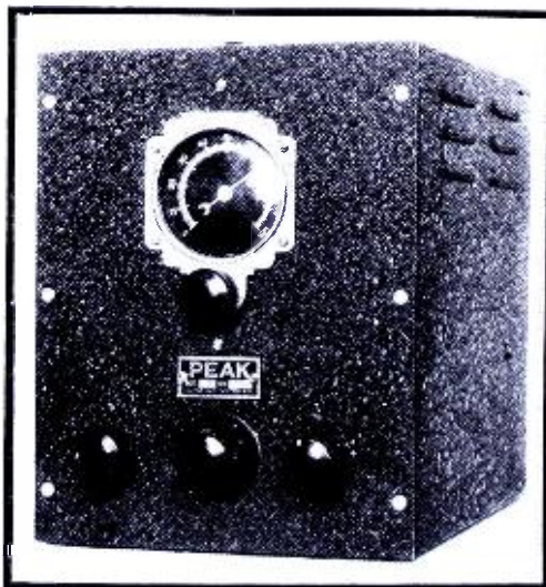
View of the preselector described here. The regenerative stage certainly does increase the gain of the first stage.
